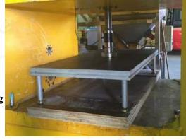
A series of tests on five Transtage All-Terrain staging units measuring 2000x1000x380 mm in height were undertaken for your company in May 2015. The tests involved the application of either a vertical point load, or a vertical uniformly distributed load to the central 1000x1000 mm part of each unit, on the horizontal surface of each unit up to a maximum deflection of 180 mm. The results are summarised below.
