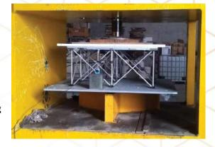
A series of tests on five Transtage Premiere staging units measuring 1000x1000x420 mm in height were undertaken for your company in January 2013. The tests involved the application of a vertical uniformly distributed load to the horizontal surface of each unit up to a maximum deflection of 90 mm. The results are presented in full in TSE *Report 248*, "Laboratory Investigation of the Load Capacity of Transtage Premiere Staging Platforms", and the load capacities are summarised below.
