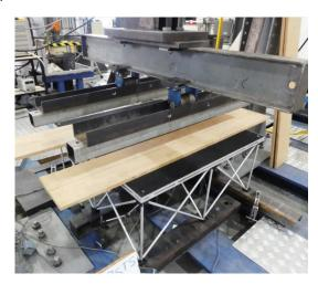
The samples demonstrated sufficient ductility and strength, withstanding the ultimate limit state pressure for over 15 minutes without visible damage. These tests confirmed compliance with the serviceability deformation limit of span/180 and satisfied the acceptance criteria for strength in AS/NZS 1664.1. For more information, please refer to the STL-TR-25-02 test report.
