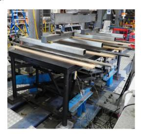
The samples demonstrated sufficient ductility and strength, withstanding the ultimate limit state pressure for over 15 minutes without visible damage. These tests confirmed compliance with the serviceability deformation limit of span/180 and satisfied the acceptance criteria for strength in AS/NZS 1664.1. For more information, please refer to the STL-TR-25-02 test report.
